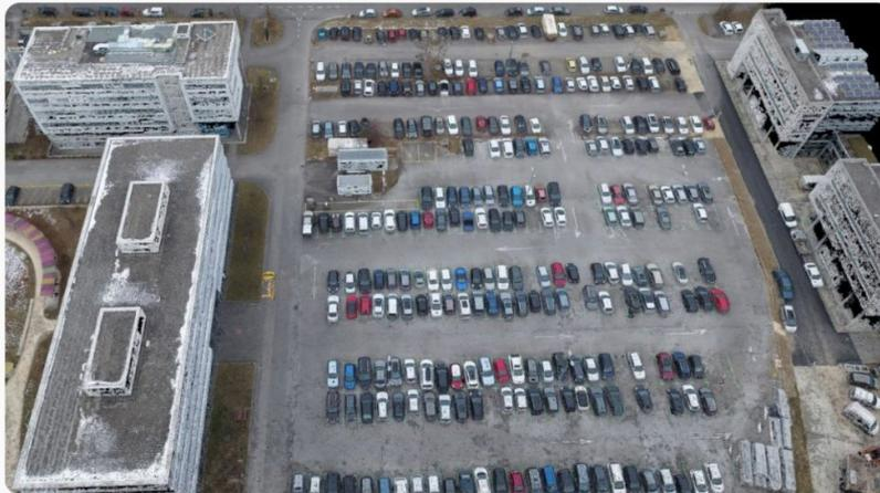
The color point cloud uses RGB data from a raster for colorization. Each point of the point cloud receives the RGB value of the raster pixel that has the same location.
